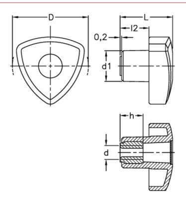
$\begin{array}{ll} d &= 40 \\ d1 &= 16 \\ d \, 6H = M8 \\ L &= 30 \\ l2 &= 17 \end{array}$
